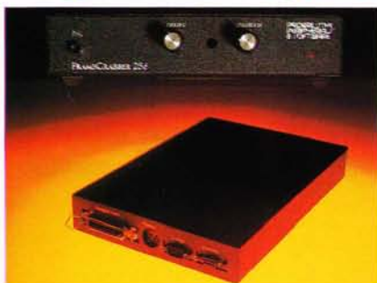
The Marcam frame grabber has manual controls, excellent software, but a price tag of £500.
